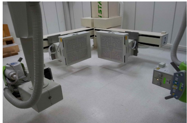
Fig. 1 Beamlines setup used for the dynamic RSA evaluations of the patients
