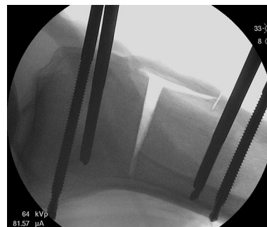
Fig. 1 Osteotomy procedure: the X-ray shows the 10^\circ wedge of the anterior proximal tibia, which was cut and secured with an external fixator, which enabled closing of the osteotomy while the specimen fixed in the testing machine
