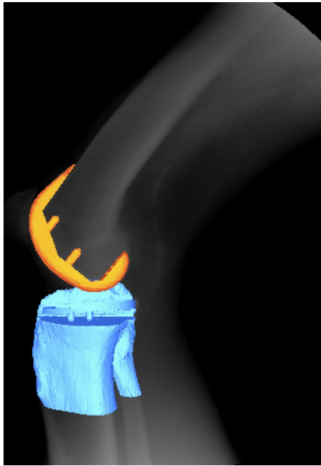
Fig. 3 Femoral and tibia/fibula/baseplate 3D models were registered to their projections in a series of fluoroscopic images to measure 3D knee kinematics
