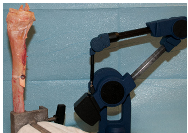
Fig. 1 Representation of the testing set-up with the knee securely positioned in a custom clamp to prevent any movement during testing. The coordinate measuring device ( in blue ) was used to measure interspatial relationships between the anterior meniscus root attachments and ACL native footprint and reamed tibial tunnels
