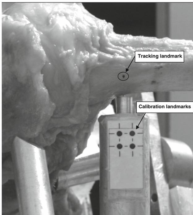
**Fig. 2** View from the CCD camera measuring the postero-anterior displacement of the proximal humerus during loading. Landmarks were placed on the humerus and on the loading device for calibration purposes
