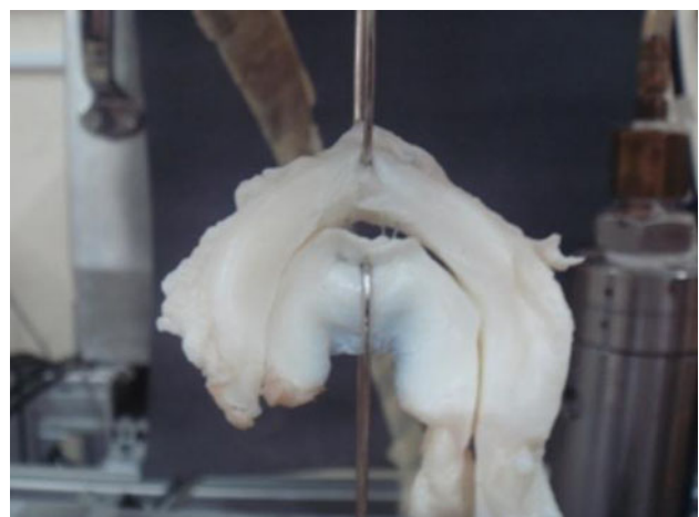
Fig. 2 Meniscal specimen undergoing load to failure testing
