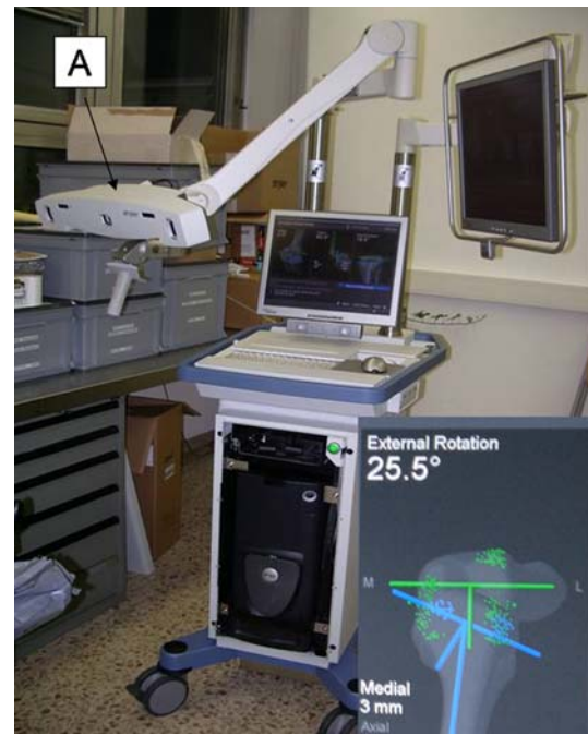
Fig. 1 The PrecisionN knee navigation system (Stryker Medical Systems, Duisburg, Germany) can measure the 3D kinematics of the knee using an infrared three-camera system (A) which can appoint the infrared trackers at the tibial and femoral bone. The measured rotation is shown on the navigation system screen
