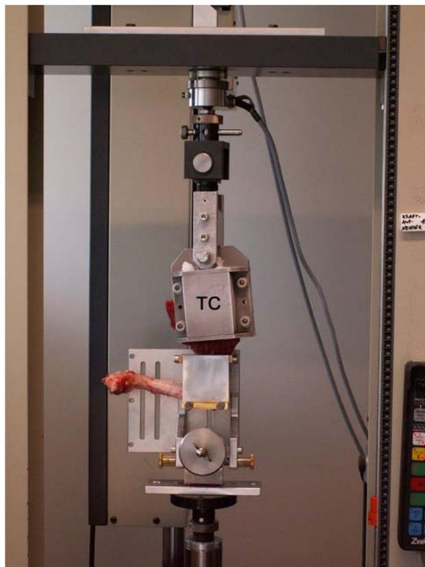
**Fig. 3** Material testing machine (Zwick 1445, Zwick-Roell, Ulm, Germany): the proximal end of the infraspinatus tendon is set in a tendon clamp (TC), leaving approximately 6 cm between the clamp and the site of repair
