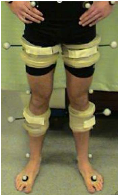
Fig. 1 Reflective marker orientation for 3-D motion analyses (posterior calcaneus and sacral markers not shown)
