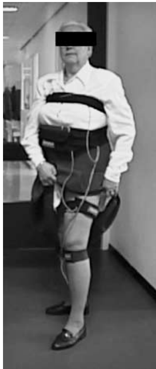
Fig. 1 Test person carrying the measurement system for the DynaPort knee test. The belts contain accelerometers
