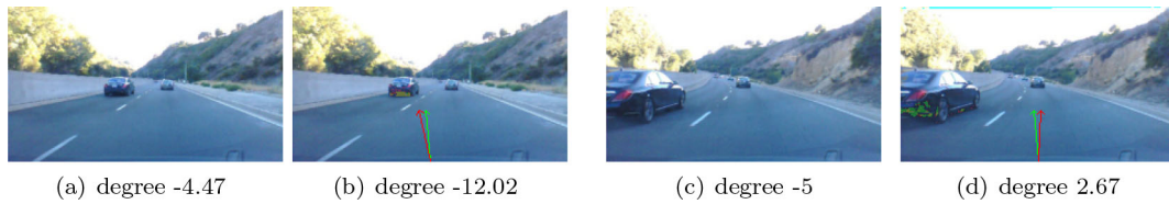
Fig. 7. Adversarial examples for the end-to-end network for self-driving cars trained on the driving dataset by single-path search
