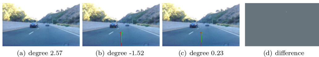
Fig. 9. An adversarial example for the end-to-end network for self-driving cars trained on the driving dataset by multi-path search
