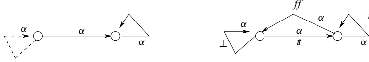
Fig. 1. On the right: a 3-valued transition system with two states and a set Act = \{\alpha\} of possible events. On the left: the corresponding interpretation which shows only may -transitions R^c \setminus R^a (with value \perp on the right, dashed lines in figures) and solid must -transitions R^a (with value \# , solid lines in figures); “transitions” with value ff are omitted
