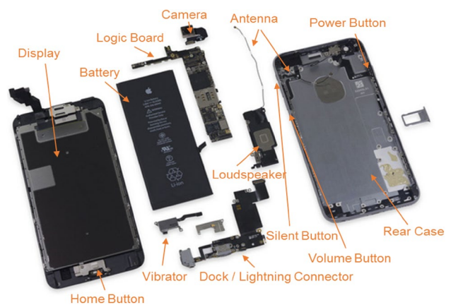
Fig. 4 Example of smartphone assemblies (iFixit 2015)
