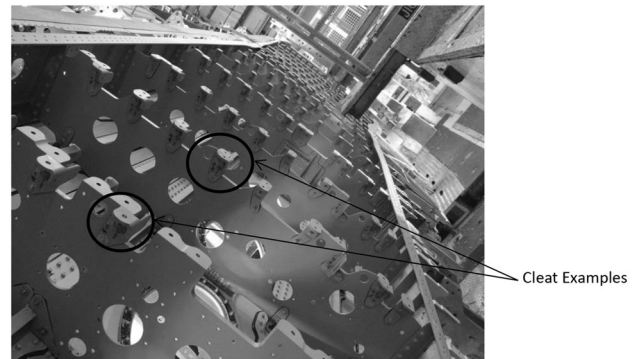
Fig. 2 Showing Butterfly brackets bolted onto wing ribs
