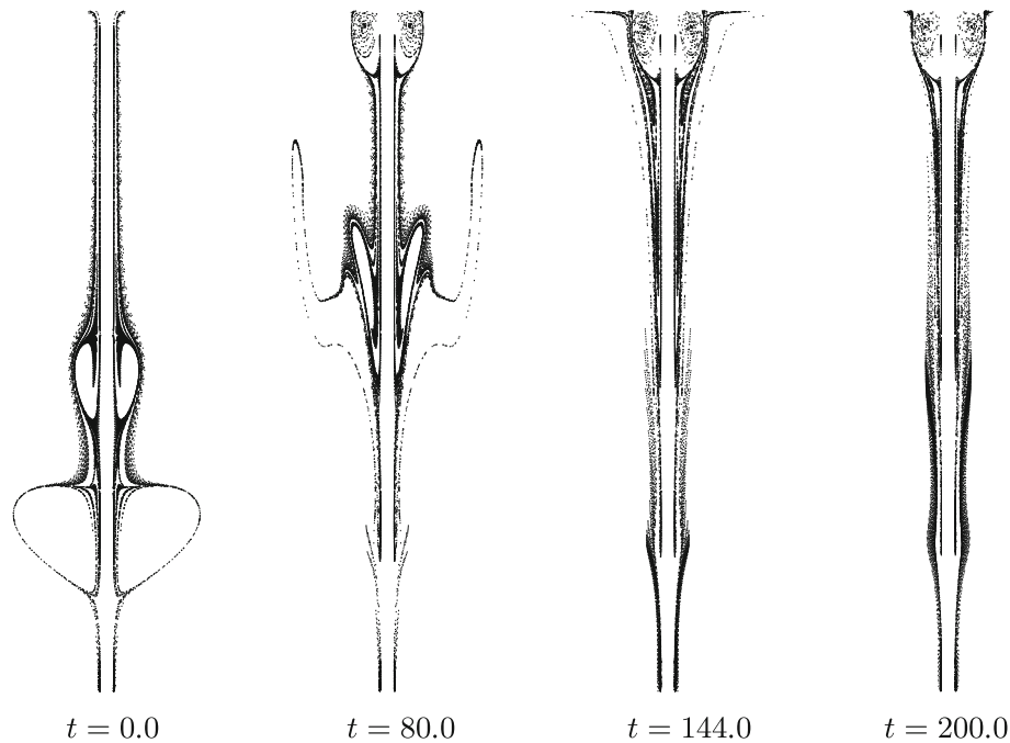
Fig. 5 Simulated visualization of the transient flow at Re_{\text{lid}} = 2200 for a suddenly started rotation of an initially fixed rod with \gamma = 0.008 , showing that the breakdown bubbles move up and dissipate in the boundary layer of the lid
