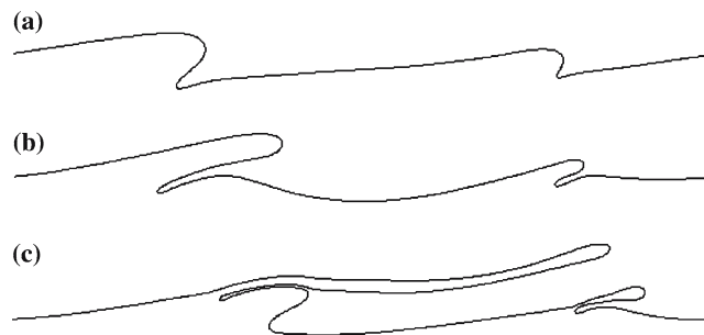
Fig. 14 Three stages of ligament formation and elongation at low Reynolds number, 512 \times 512 grid, case C Re_g = 500 and We_g = 4,000 , a t = 4 , b t = 5.6 , c t = 8.8
