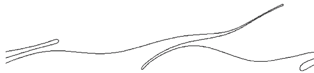
Fig. 21 Case D1 (the same as D but at a larger perturbation amplitude): the breakup occurs much earlier, just after time t = 4 , which is shown here
