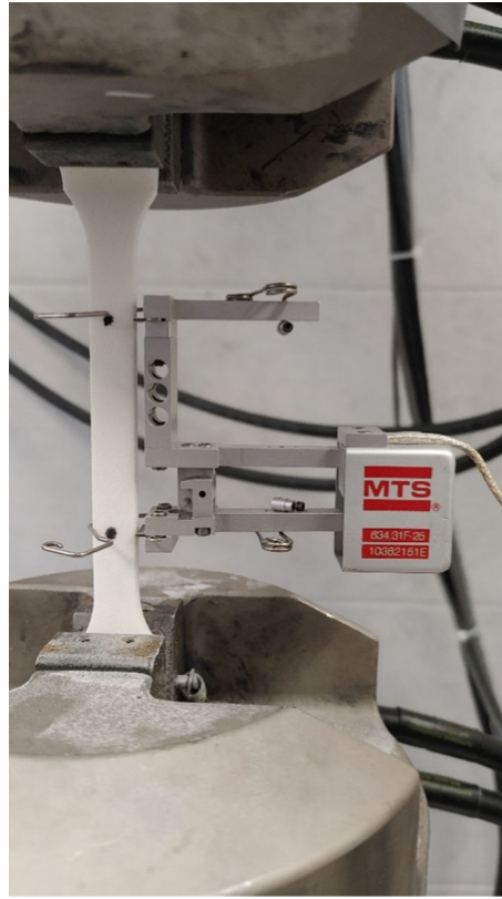
Fig. 3 Test setup to obtain tensile stress–strain responses of the specimens
