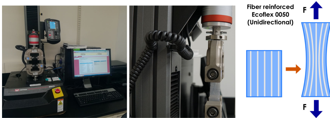
Fig. 11 Experimental set up (left): uniaxial tension test of elastomeric composite (50 mm \times 25 mm); schematic illustration of the uniaxial strain of the reinforced elastomer (right)
