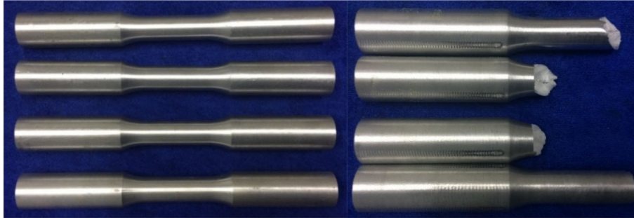
Fig. 8 Specimens for fatigue test
