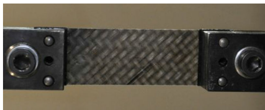
Fig. 45 Clamping device for the 36 mm specimen in the undeformed configuration
