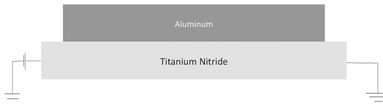
Fig. 4 Schematic of the Blech structure that was used in the simulation
