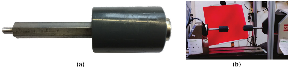
Fig. 5 Visualization of the axial force measurement. a A magnet in a plastic holder, connected to an aluminum distance rod. b Measurement of the forces with a microtensile testing machine
