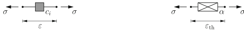
Fig. 4 Dissipative strain element with material parameters c_i (left), thermal strain element with expansion coefficient \alpha (right)
