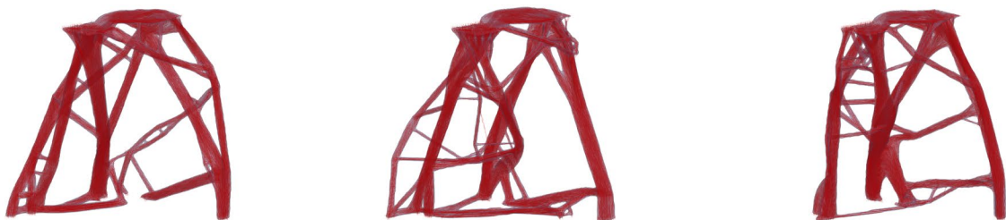
(d) Fiber orientation, TFP-X (e) Fiber orientation, TFP-Y (f) Fiber orientation, TFP-Z
