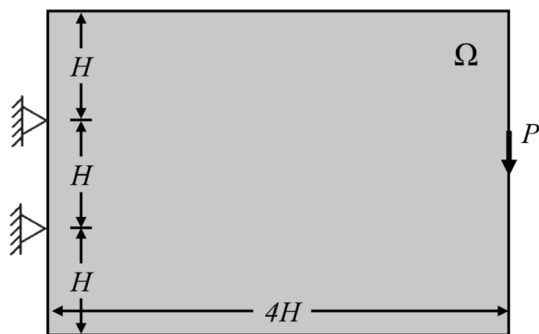
Fig. 8 Michell beam design domain and boundary conditions
