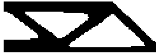
(b) Upscaled and projected MBB-beam to a 120x40 FE-mesh w. compliance 191.1536 (compared to 191.2364 in Zhang et al (2021b)).
