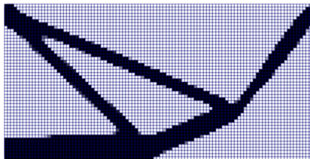
Fig. 5 Topology optimization result for force inverter mechanism
