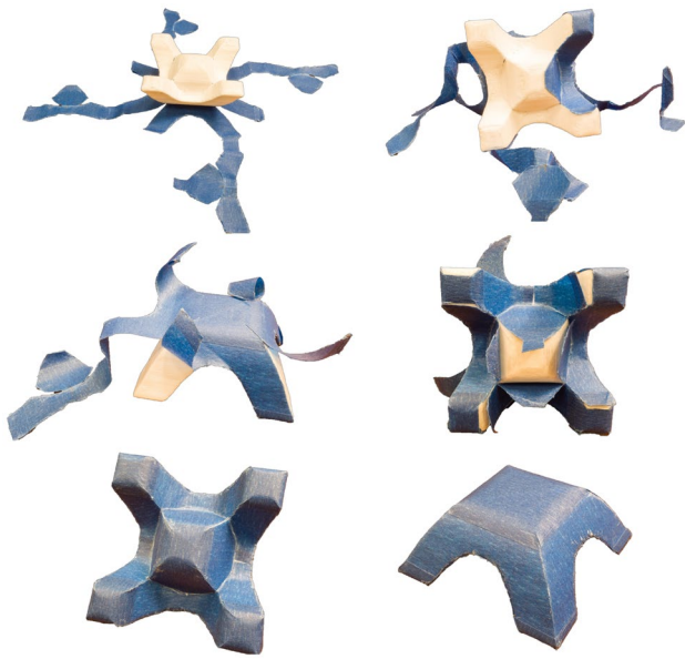
Fig. 9 The prototype demonstration of taping a 2D pattern to the surface of an optimized and printed solid volumetric part
