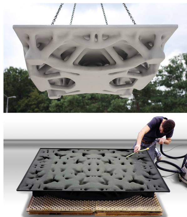
Fig. 13 From top to bottom: Topology optimized slab (Credits: Andrei Jipa, Digital Building Technologies, ETH Zurich) and respective sand formwork (Credits: Benjamin Dillenburger, Digital Building Technologies, ETH Zurich)
