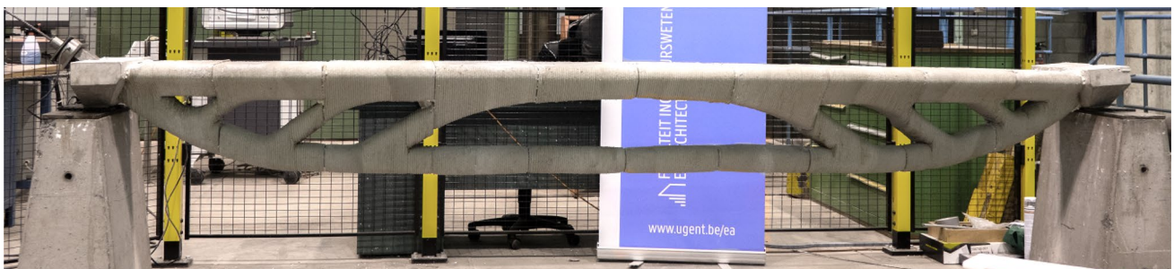
Fig. 14 Topology optimized 3D printed, post-tensioned concrete girder investigated by Vantighem et al. (2020) (Credits: Gieljan Vantighem, Faculty of Engineering and Architecture, Ghent University)
