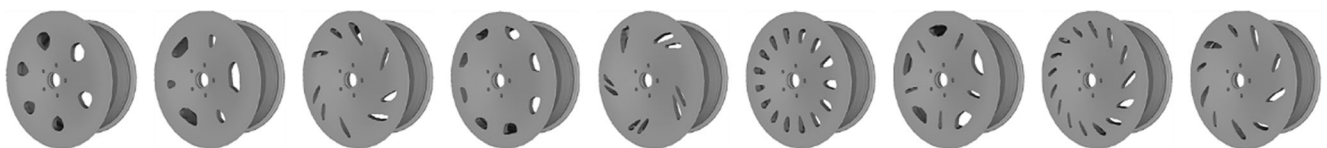
Fig. 21 Wheel design candidates in the order of highest stiffness (from left to right)
