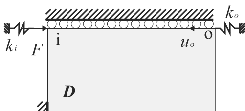
Fig. 16 The design domain of the displacement inverter
