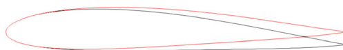
Fig. 7 Optimization results for 6 mm constraint, undeformed (black) and deformed at Mach 0.5 (red) configurations
