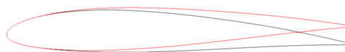
Fig. 6 Optimization results for 10 mm constraint, undeformed (black) and deformed at Mach 0.5 (red) configurations
