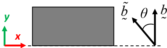
Fig. 2 Rotation of the reference build direction vector, b , to the transformed build direction vector, \tilde{b} , by \theta . Build plate omitted for clarity
