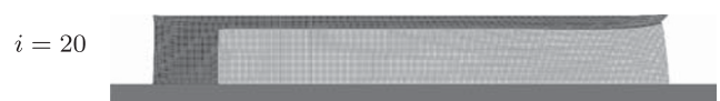
Fig. 8 Displacement plot of the cantilever example with a mesh resolution of n = 300 \times 40 = 12000 elements
