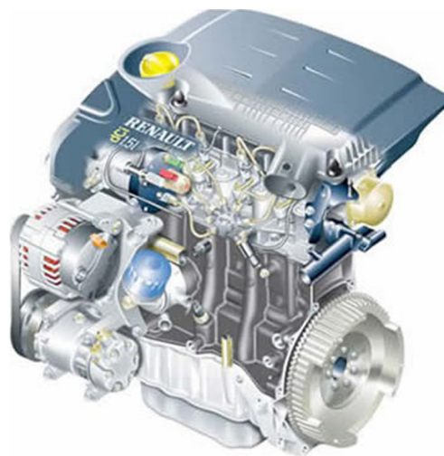
Fig. 2 Reference engine (belt, accessories and bracket are in the lower left-hand corner)
