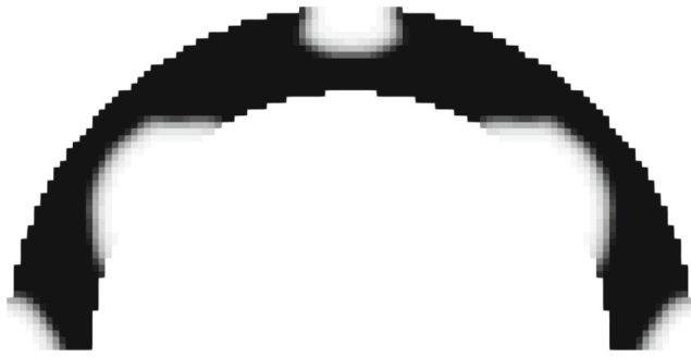
Fig. 16 Optimized design with the density-based topology optimization. The objective value of the end design evaluated with mixed formulation, C = 0.0022N
