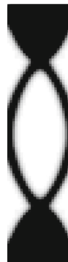
Fig. 9 Optimized design with the density-based topology optimization. The objective value of the end design evaluated with mixed formulation, \mathcal{C} = 48.9N
