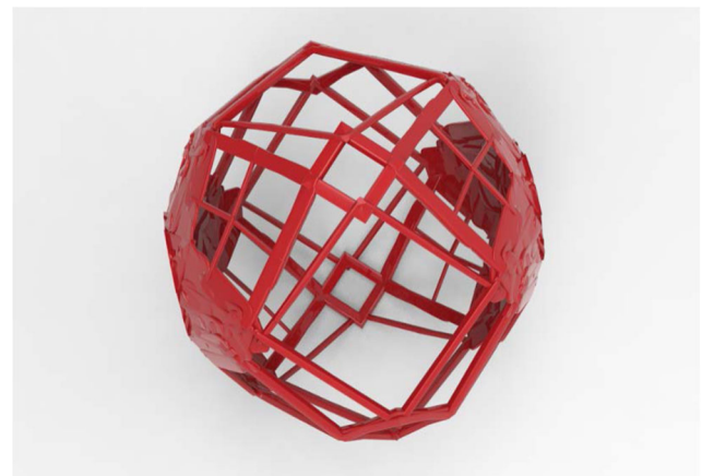
Fig. 26 The CAD model of the optimized structure obtained by the proposed method ( \bar{V} = 0.02V_D , 126 \times 105 \times 126 background elements and 42 \times 35 \times 42 analysis-elements)
