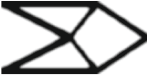
Fig. 8 Optimal topology for static load
