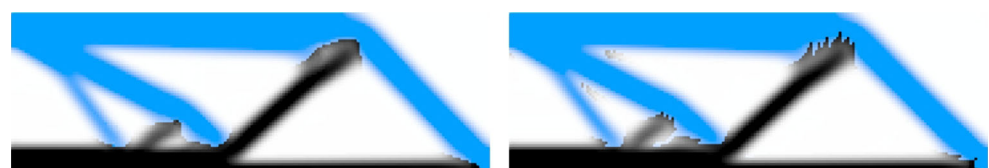
Fig. 3 Results for the Messerschmidt-Bölkow-Blohm (MBB) beam with sensitivity filter (left) for phase variable and without (right)
