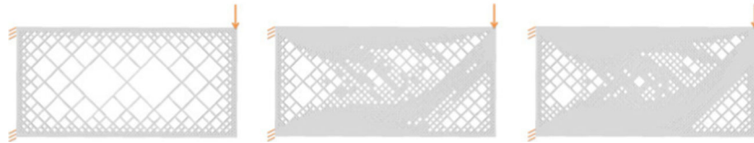
(b) The self-support rhombic cell infill (Wu et al. 2016), from left to right: the initialization, result of 70% material fraction, and result of 78% material fraction
