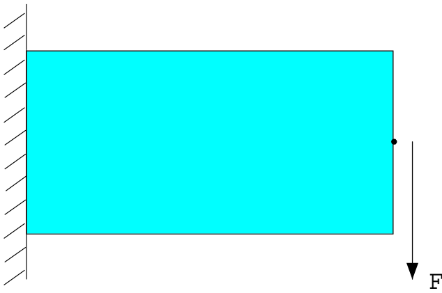
Fig. 1 2D cantilever beam.
