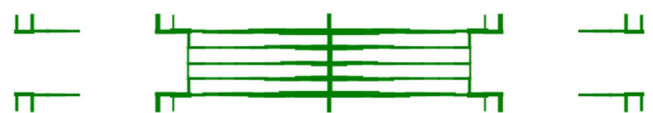
Fig. 12 Optimized result with HCATWS-2 for 3P crash case 1 (outer walls not shown)
