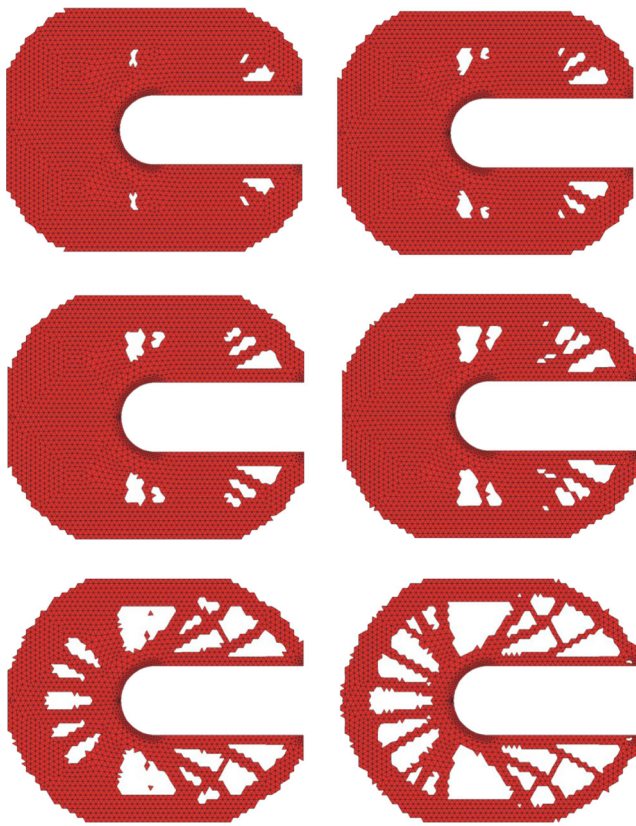
Fig. 13 The C-shaped structure. Selected intermediate (iterations 10, 15, 20, 25, 35) and final (iteration 40) topologies
