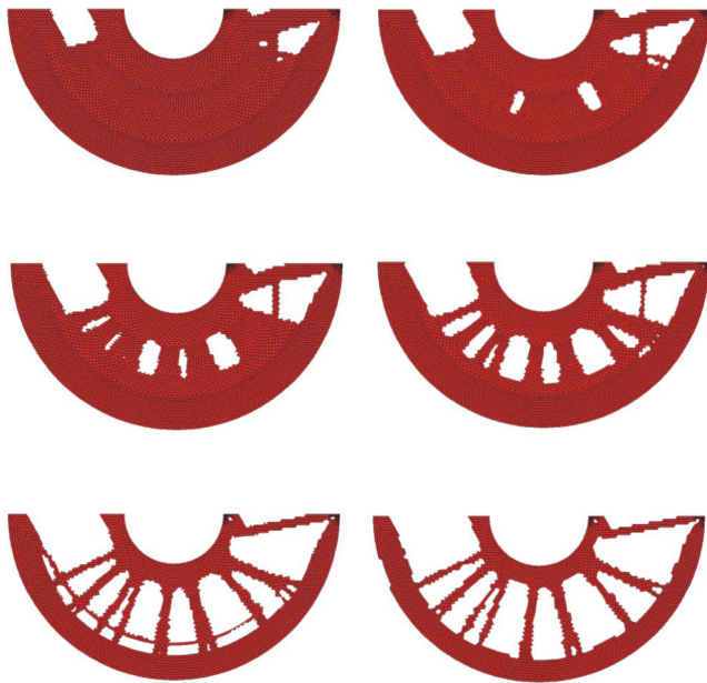
Fig. 37 The half-ring structure. Selected intermediate (iterations 10, 30, 40, 50, 60) and final (iteration 80) topologies
