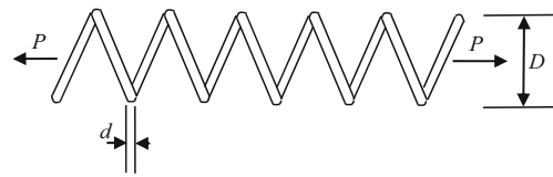
Fig. 8 The tension-compression string design problem
