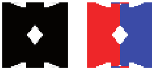
Fig. 5 Structure layout ( left ) and electrode profile ( right ) that isolate the second mode shape when considering the first 4 modes in-plane
