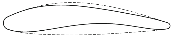
Fig. 8 The contour of the optimal blade (solid line) found by the first set of the optimization parameters \mathbf{x}_{P1} and the MM structural analysis. The reference geometry is depicted with dashed line
