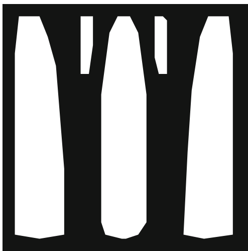
Fig. 16 A SIMP-generated design with 50 % volume fraction
