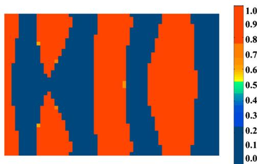
**Fig. 8** Optimal solution for the cantilever plate without model reduction
