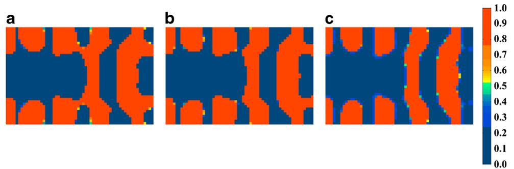
0.5 m above the plate center. Six different excitation frequencies ( $f_p = 26, 31, 42, 60, 85$  and  $130$  Hz) are considered, and the corresponding optimal designs are shown in Fig. 12. As expected, as the excitation frequency increases, the optimal layout of electrode becomes spatially more complex to suppress localized vibration modes excited by the external forces.
