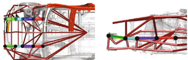
Fig. 6 Front crash substitute model. Black dots represent branching points of the middle load path
