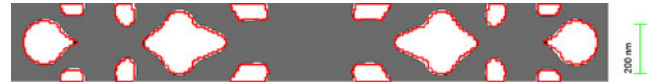
Fig. 4 Proximity effects - comparison between blueprint design (courtesy of F. Wang) obtained by topology optimization (Wang et al. 2011a) shown in red, and manufactured photonic crystal shown in gray (courtesy of Dr. Lars H. Frandsen)
